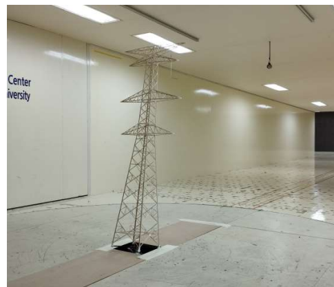
Figure 3. Tilted model in the wind tunnel.
